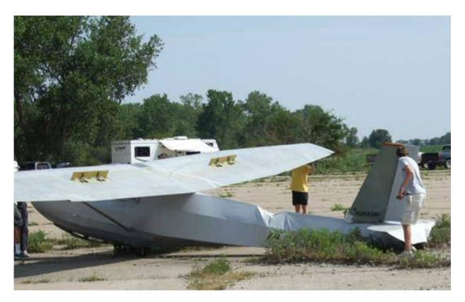
The damage is extensive to the fuselage, horizontal, elevator and the right wing root has a significant wrinkle. Not one of us could have prevented this event. Of those I talked to Debbie Smith, Dennis Brown, John Bird and Sue Erlenwein turned away from the wind and saw a 180 version of what Harry and I saw looking into the wind. I'm not sure how many other people saw the entire thing? But it hurt. And it hurt many people on that ramp who love flying things.
