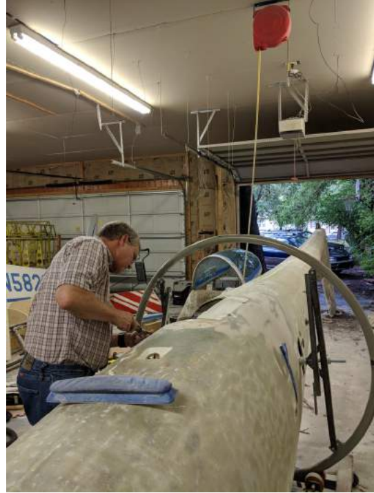
Bob Hinson works on fairing in the gear doors
