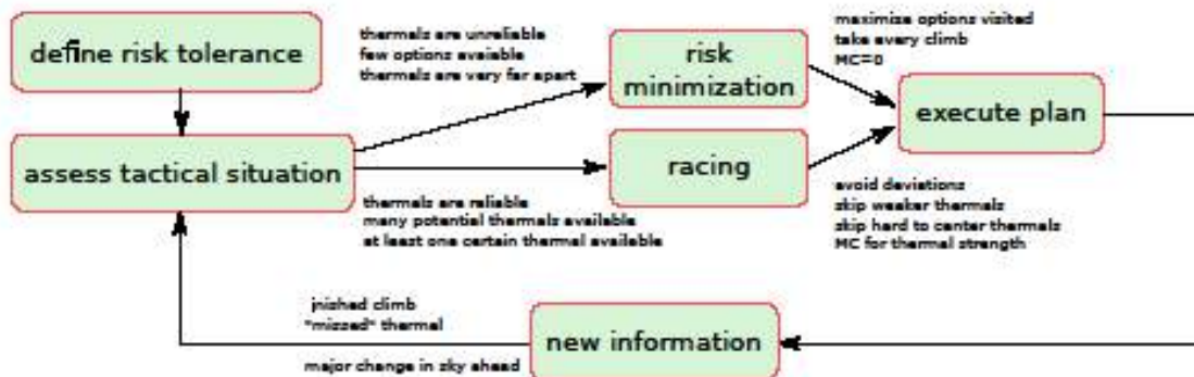
Fig. 8 Schematic describing the decision-making process for risk aware thermal soaring. Gear shifting occurs when the pilot receives new information which reveals a change in the risk situation and reevaluates the decision-making frame. This could happen for example when missing an expected climb or when reaching a “blue hole” with few clouds.
