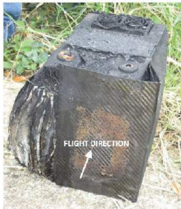
Figure 5 Fire damage to the forward FES battery
